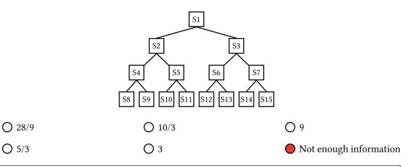
**Solution:** Not enough information, because the order of the nodes in the overlay ring, which is not specified, is crucial for calculating stretch.
